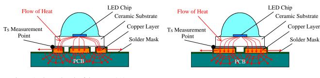
Figure 4. Thermal Path of the NVSx219C LEDs
